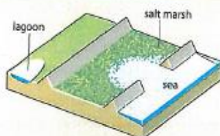
Figure 18.26 Breaching of an old sea-wall to create a salt marsh
