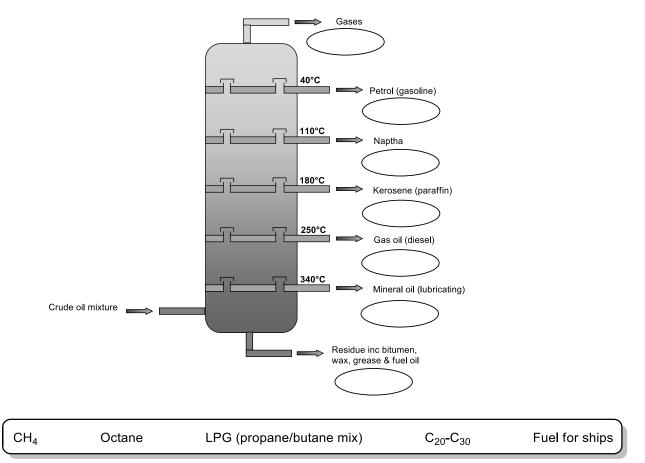
**1.** The diagram shows a fractioning column.
